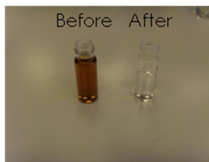
Figure 2. Comparison of the solution obtained before and after using AFFINIMIP® SPE Bisphenols
