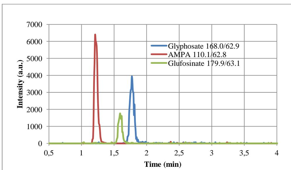
**Figure 3.** LC-MS/MS chromatogram obtained for the three main ion transitions for glyphosate, AMPA, and glufosinate from a sea water sample spiked at 200ng/L and purified using **AFFINIMIP® SPE Glyphosate**.
