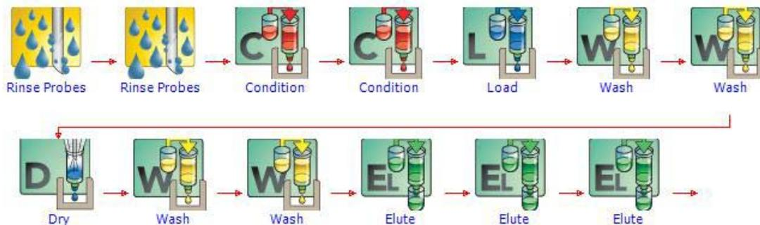
**Figure 3.** TRILUTION LH SPE Tasks for Extraction of Zearalenone (ZON) from Wheat Extract
